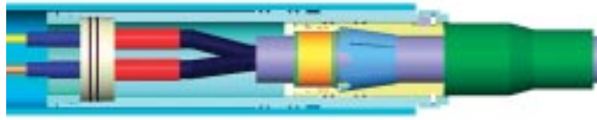
Fig. 1. Field Assembled Cable Termination (FACT) Penetrator with high-pressure “Web” that isolates the cable from the pressure-balanced splice chamber
