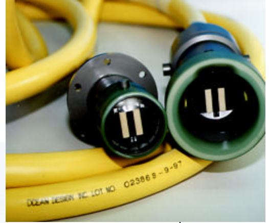
Cable-end Connectors showing End seals
