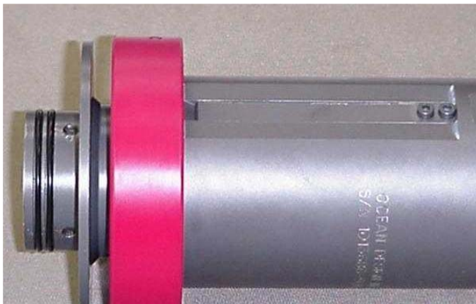
Photo 1: ROV Connectors showing ROV Latch Fingers in the closed position
